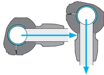
For rigid drops with horizontal take off or for all types of air supply with rigid pipe or flexible hose on an installation which incorporates an efficient air dryer.
