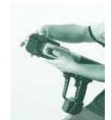
Lock in position by closing the retaining pin.
