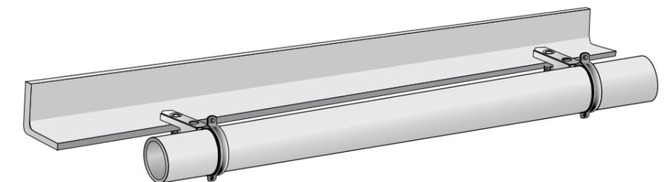
Position the clamps ref. ER99 onto the RSJ or beam in accordance with the minimum recommended number of attachments per length of pipe and the required distance between attachments, according to the diameter of the pipe.
