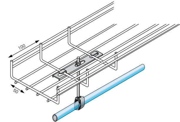
Use the under-cabletray attachment ref. 6699 10 30 and suspend with threaded rod up to M10 diameter. This attachment can be used to suspend networks from Ø16.5 to Ø100.
