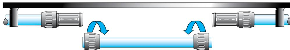
Loosen the nuts located on the side of the pipe to be removed and slide them along the pipe. Then remove the pipe.
