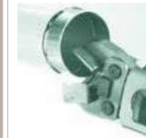
Manually open the jaws of the clamp and insert the stainless steel pipe into the clamp as far as it will go.
