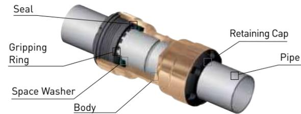
Pipe-to-pipe and stud connectors in Ø22 and Ø28 can be immediately connected to Transair® stainless steel pipe – simply push the pipe into
