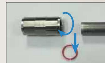
Disassembly : 5. Re-screw the nut on the fitting without the red ring; it is ready for assembly.
