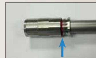
Disassembly : 2. Put the red dismounting ring on the pipe and re-screw the nut on the fitting.
