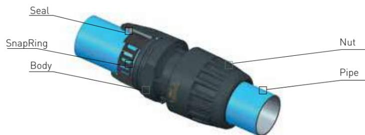
Ø50 and Ø63 connectors are quickly secured to Transair® aluminium pipe by means of a SnapRing which makes the connector fully integrated with the pipe.
