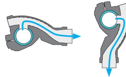
New generation quick assembly brackets are recommended for vertical or horizontal take-offs, using either rigid pipe or flexible hose.
