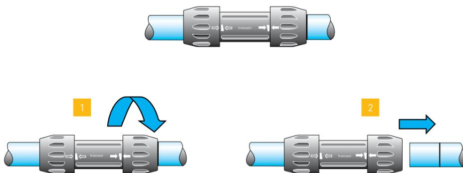
Simply insert the pipe into the connector up to the connection mark.
