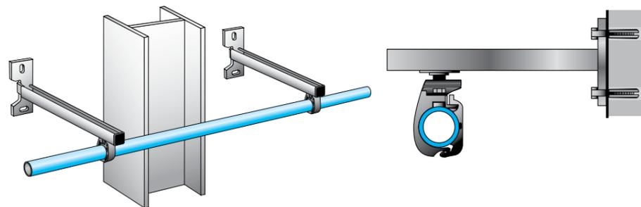
Transair® U-channel assemblies are used to offset networks and to bypass obstacles. They comprise sectional rail ref. 6699 01 01 and a series of attachment accessories 6699 01 02.
