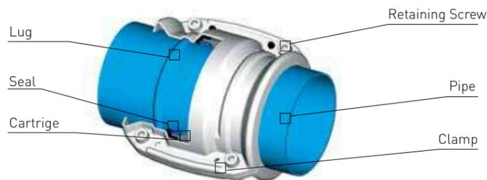
Ø76, Ø100 and Ø168 clamps secure instantly to Transair® aluminium pipe. Simply position the formed pipe within the Transair® cartridge, which acts as a seal.
