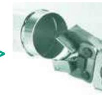
Re-open the two jaws to remove the pipe and rotate the pipe slightly.
