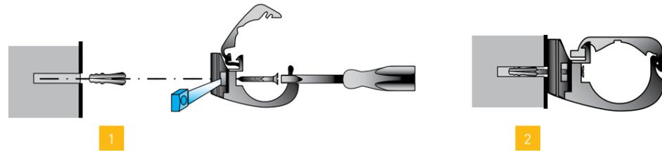
1 - Remove the nut at the base of the pipe clip using a screwdriver. Insert the screw by passing it through the clip.
