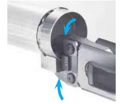
Release the jaws. Press the trigger and crimp the tube until a 'snap' sound is heard.
