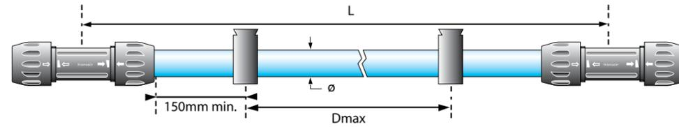
The Transair® fixing clip is the basic component for mounting pipe when installing. Ø16.5-Ø25-Ø40-Ø50-Ø63 Transair® aluminium networks. Only this clip should be used since it allows expansion and contraction of the pipe to occur freely.
