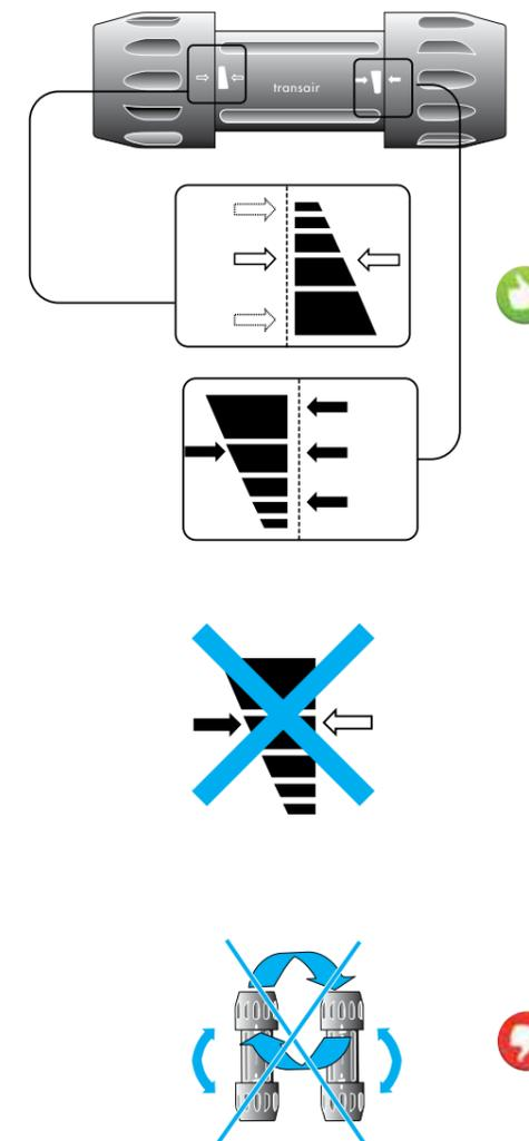
There is no need to loosen the nuts prior to joining Ø16.5, Ø25 and Ø40 connectors to Transair® aluminium pipe. **Do not exchange the nuts.** **Do not use a nut on another connector.**
