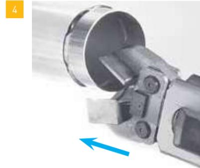
Manually open the jaws of the clamp and insert the aluminium pipe into the clamp as far as it will go.
