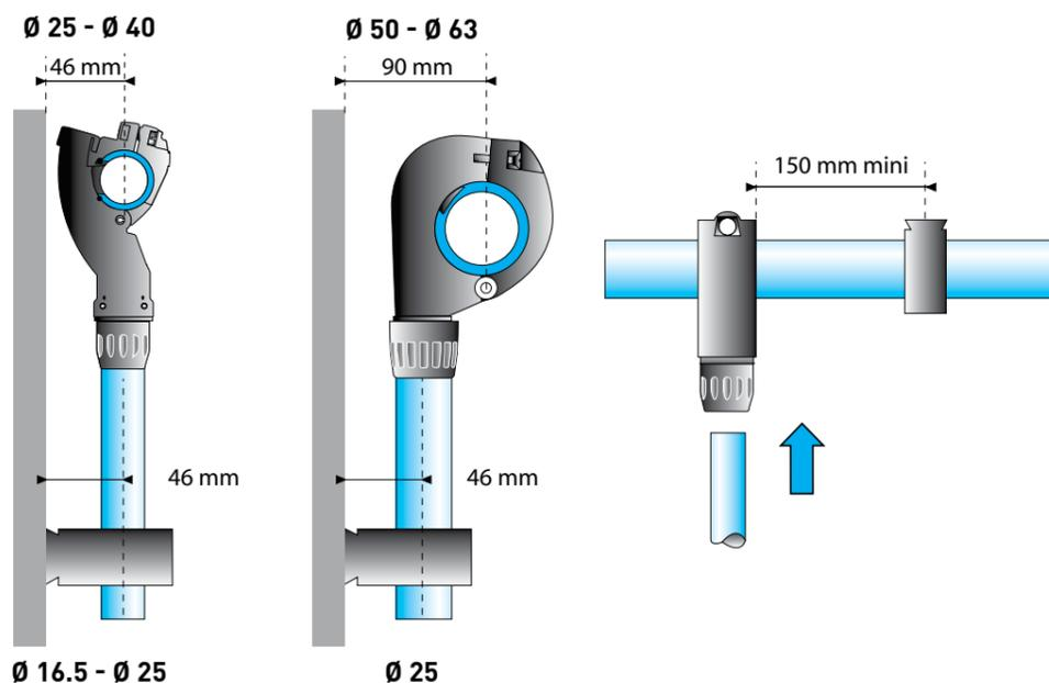
For Ø25 and Ø40 Transair® quick assembly brackets, the pipe centre to wall distance is equal to the bracket centre to wall distance, i.e. 46mm.
