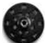
Sanding pad With hook and loop fastening, Ø 150 mm with M 14 suction hole. Hole circle suitable for FEIN and other sanding materials.
