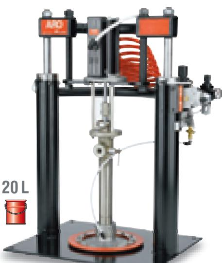
**22:1 ratio extrusion packages for 20 L drum**
