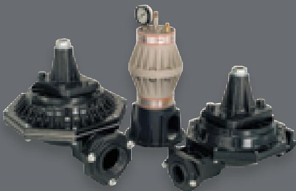
**Pulsation Dampeners:** ARO Shock Blocker® pulsation dampeners are installed in fluid transfer / supply operations to avoid material pulsation and foaming. Pulsation dampeners also help reduce "hammering" or stress on fluid piping that can occur when reciprocating pumps are operated at slow or intermittent cycle rates.
