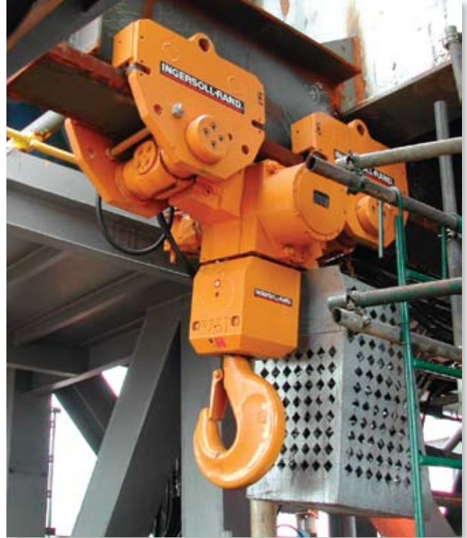
BS75LCA3 (75-ton) air system – 1 hoist shown
