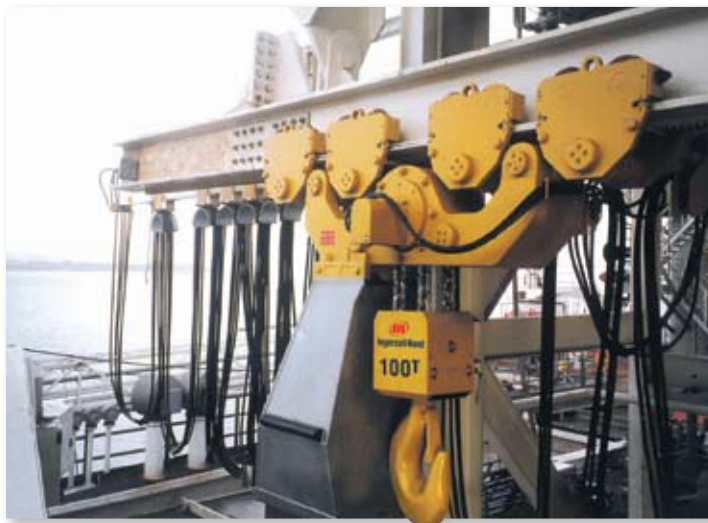
Liftchain® 200-ton BOP Handling System (1 hoist shown)
